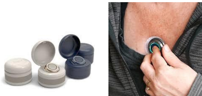
Figure 2 The CUE1+ device may help improve motor and non-motor symptoms in people with Parkinson's using a non-invasive approach. It is a discreet device (40 mm diameter, 11 mm height, 17 g) and attaches to the sternum with dermatologically tested adhesive patches. Water-resistant but not waterproof, it should be removed before showering. When active, it uses a silent motor to provide focused vibrotactile stimulation, following a specialised pattern based on extensive user testing and clinical research. It combines low frequency auditory cueing with high frequency focused vibrotactile stimulation through its distinct wave shape and frequency patterns. The CUE1+ sham device has the same exact appearance, but its treatment settings have been deactivated for the purposes of the study.
