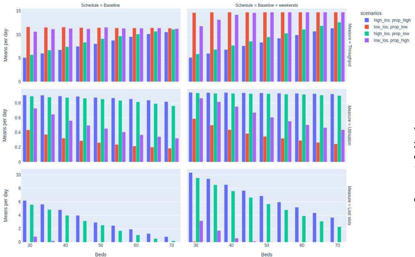
Figure 2 Results of simulations across 30–70 beds, for each of 2 theatre schedules with 4 combinations of lengths of stay (baseline:high LOS; baseline \times 0.25: low LOS) and proportion delayed (baseline:prop_high; baseline \times 0.25: prop_low) for mean daily total surgical throughput, bed utilisation and lost slots.
