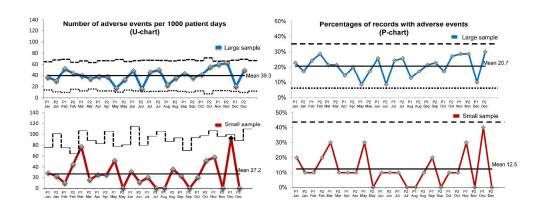
Comparison of statistical process control charts (U-chart) and (P-chart) between large and small sample. ---= Upper control limits, --= Lower control limits  $297 \times 210 \text{mm} (300 \times 300 \text{ DPI})$
